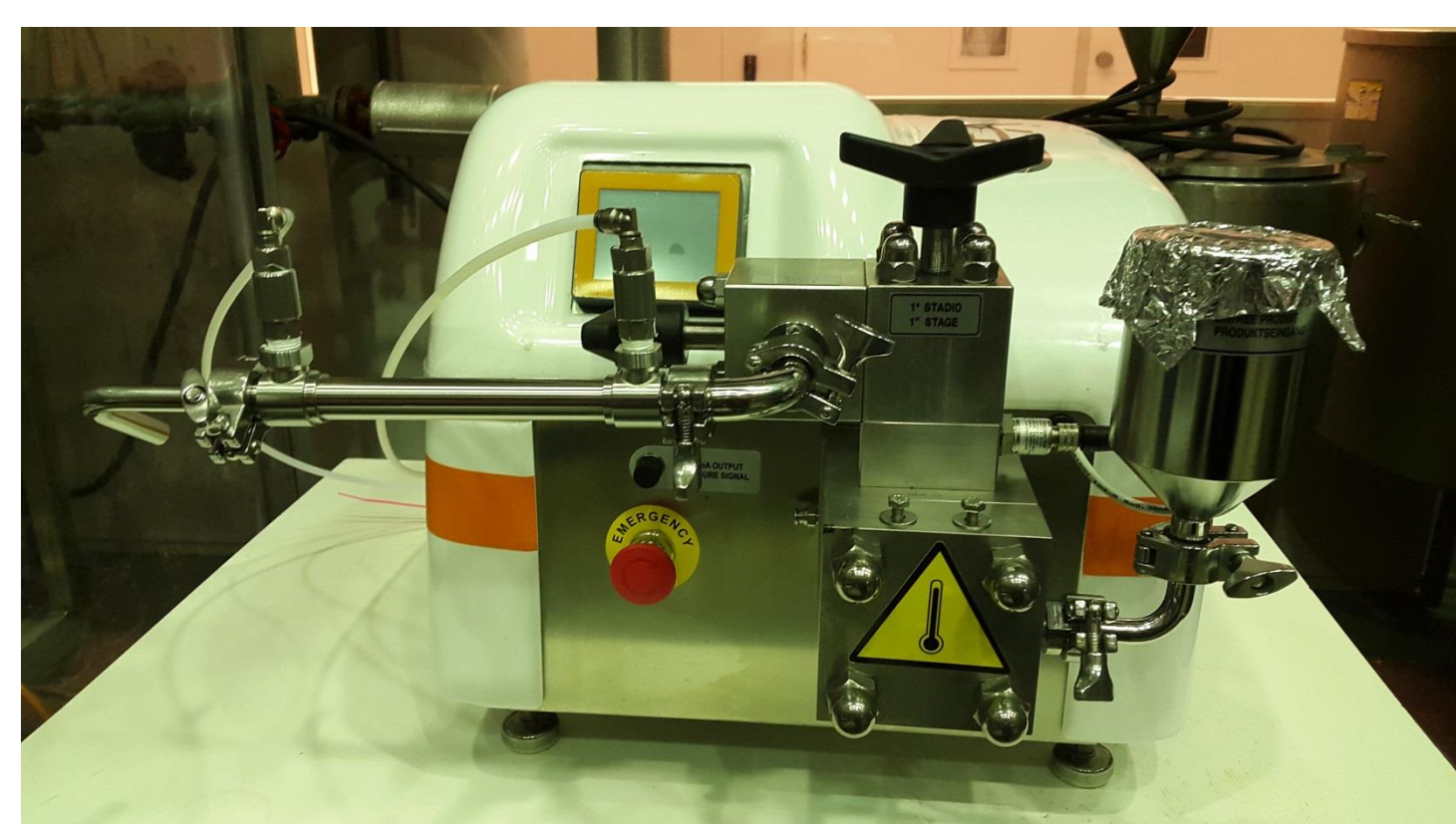
Figure 1. Bead mill (A) and high pressure homogenisator (B).
