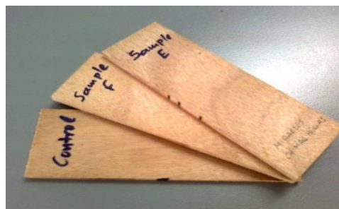
Plywood panels produced with reference PF & PF-algae resins (samples F & E)
