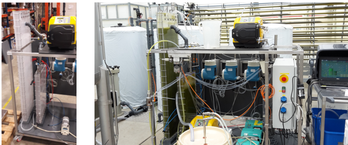
Figure 9. Continuous MAF-device (LEFT) integrated in the Sunbuilt algae pilot plant (RIGHT) at the TMC facilities.
