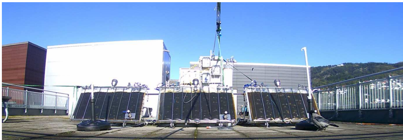
Figure 4: The GWP III systems on the roof of the UoB building in Bergen with the three P. tricornutum strains
